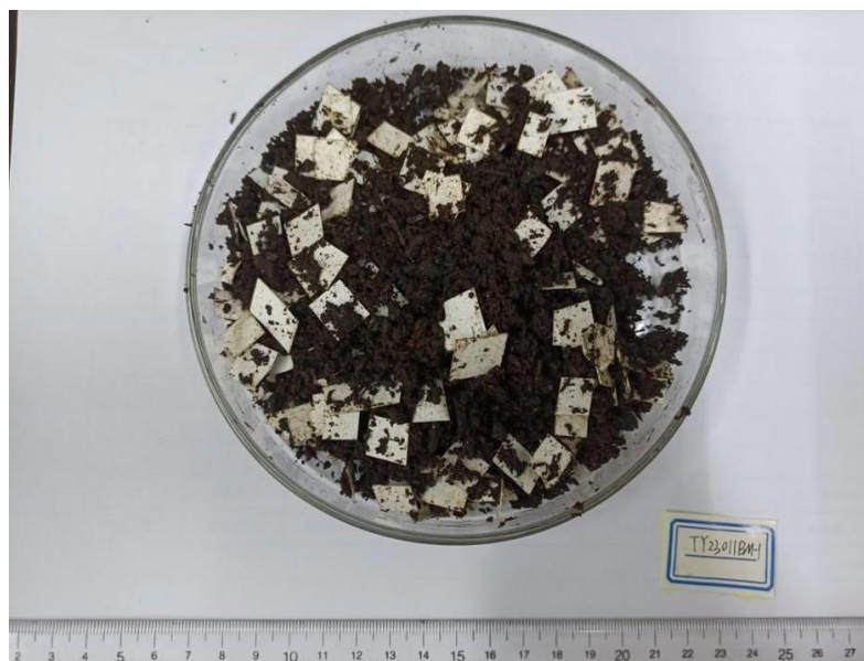
Fig.10. The picture of 721679644-2 and compost before test (mat -1)
